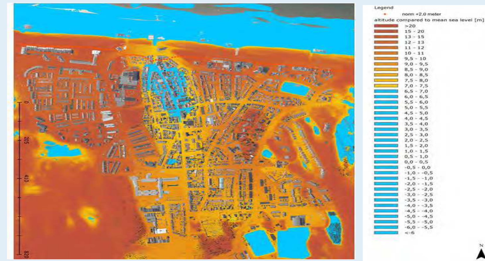
Figure 1: Predicted flooding for 2m sea level rise in case of a storm surge.
